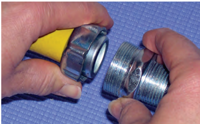
Figure 4. Shielded flexible conduit is designed to be compatible with commercial liquidtight flexible conduit fittings, which provide shield-to-ground (shield-to-drain) connections when terminated as designed to a bulkhead or metallic enclosure.
